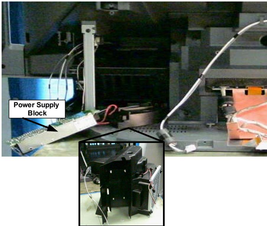
4 Grasp the Fan assembly and pull out to remove.
