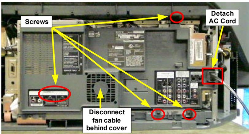
2 Remove 5 screws and detach AC cord from the slot. Pull sub plastic cover **slowly** straight back and off.
