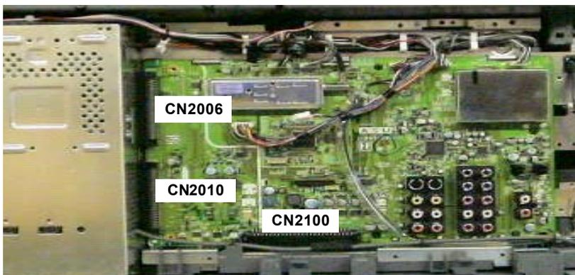
4 The ASU-Board can be probed for troubleshooting at this point of the disassembly process. It can not be remove at this point. Reference "ASU & G-Board Removal" section.
