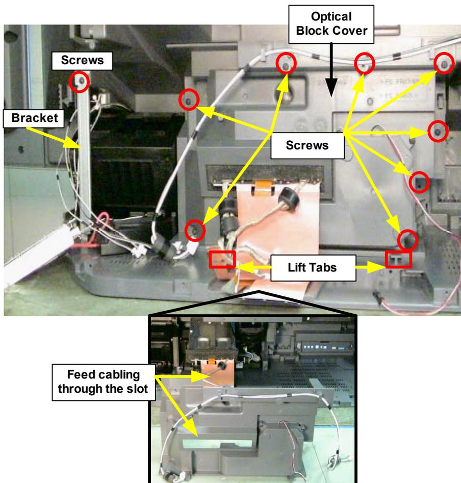
5 To access the Optics Block the gray plastic cover must first be removed. Remove the 8 screws securing the Optics cover. Lift the 2 tabs, and carefully slide cover back. Also remove vertical bracket (1 screw).
