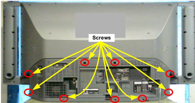
1 Remove 9 screws and pull rear plastic cover straight back and off.
