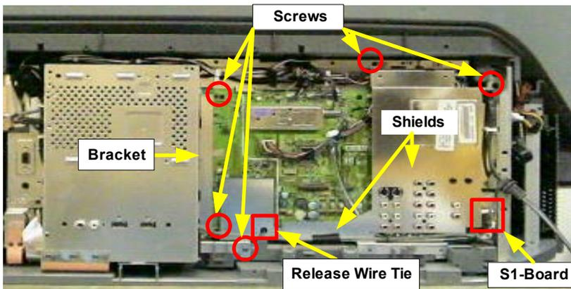
3 Remove 4 screws and release the one wire tie. Slide the bracket up slightly and pull off. Disconnect the S1-Board. Remove both shields to access the ASU-Board.
